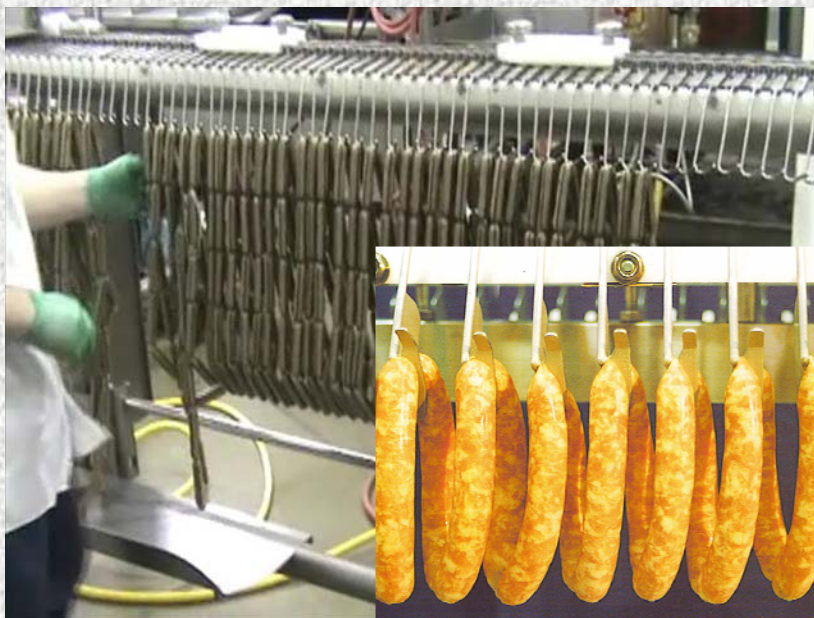
Change over from natural casing to artificial in less than 5 minutes
